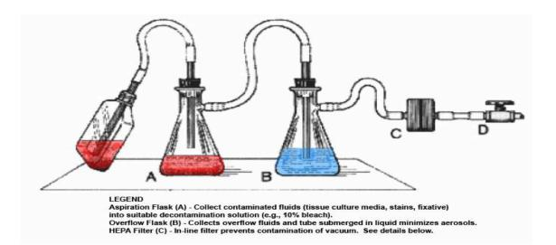
**1.** Utilizing thick-walled plastic tubing, aspirate the media from the sample flask (far left flask) to the aspiration vacuum flask (A). The aspiration vacuum flask (A) is connected to the overflow
